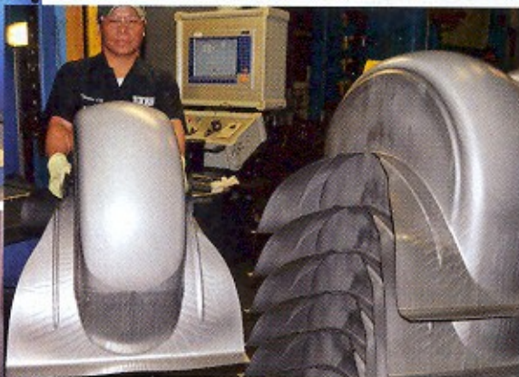
Type 304L stainless-steel blanks, 20 gauge, are deep drawn in an 850-ton AP&T hydraulic press, then laser-trimmed in a five-axis Prima cutting machine before undergoing a final restrike in a 1000-ton hydraulic press.
